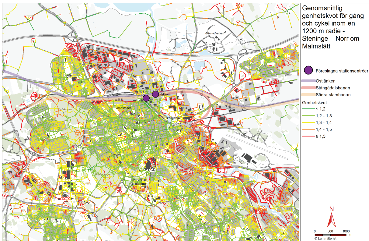
Figure 4 Example of the results of one of the BEA: Analysis for the Steninge corridor of the average detour factor for cycle and pedestrian trips within a radius of 1 200 m from each street segment. Range detour factors between \leq 1,2 and \geq 1,5 .
