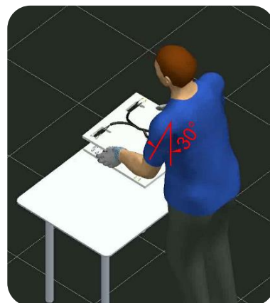
Figure 3. RULA left arm evaluation—this image is a representation of a real picture.
