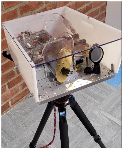
Fig. 2. Photograph of the radar system, ready to perform measurements in an industrial environment.
