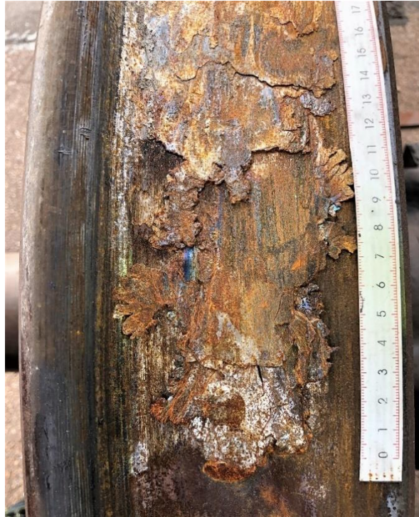
Figure 9: Material addition from brake blocks during tread braking
