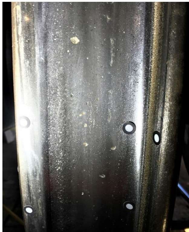
Figure 6: Wheel with indentations on the tread. The black and white dots were used as markings during the 3D scanning activities of Paper E
