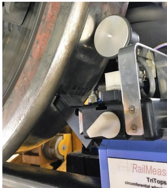
Figure 11: Measurement of wheel OOR for Paper B . The pulse wheel (upper part of the figure) and the measurement probes (centre part of the figure) of the commercial equipment TriTops can be observed [26]
