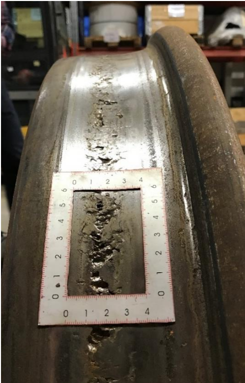
Figure 4: Wheel with severe RCF damage
