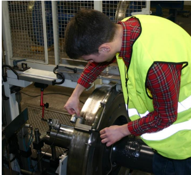
Figure 10: Measurement of the wheel profile used in the simulations of Paper B
