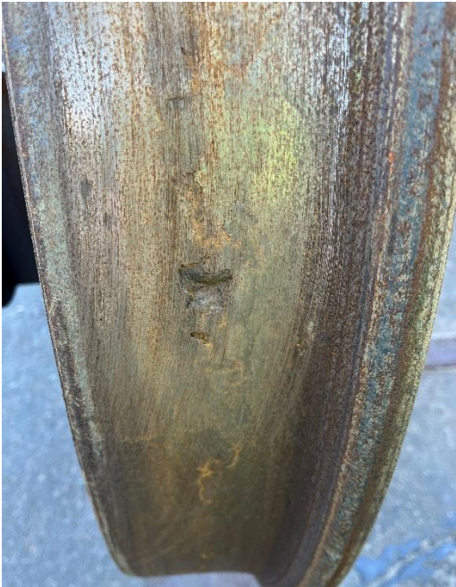
Figure 5: Wheel with isolated RCF defects
