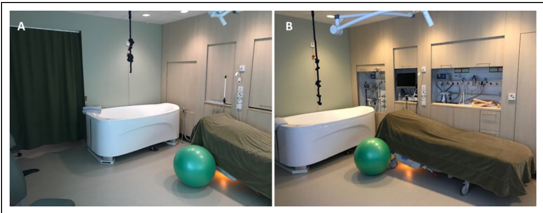
Figure 2. New birthing room where the medico-technical devices were hidden behind wood-paneled walls (A) that could be rolled up if required (B).
