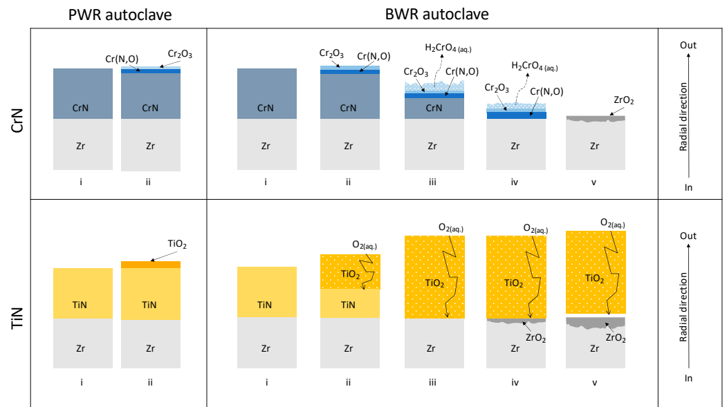
Figure 3. Schematic of the proposed corrosion mechanisms for CrN and TiN in the PWR autoclave and BWR autoclave environments.
