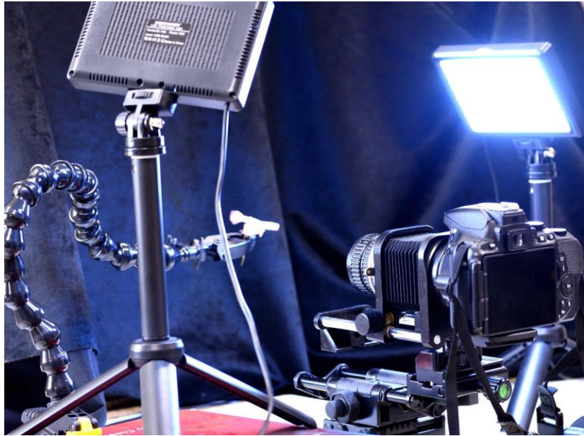
Figure 2- Macro Photographic Technique with a Bellows.
