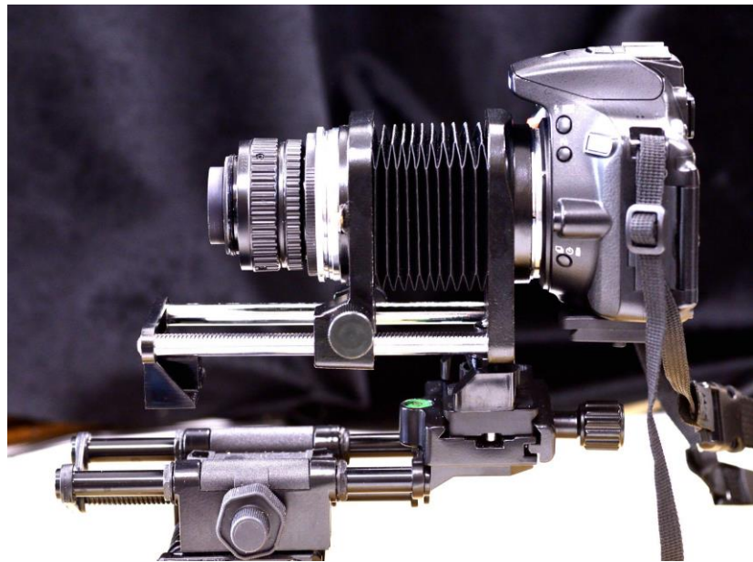
Figure 3- Macro Photographic Technique with a Bellows.
