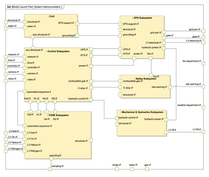
FIGURE 3 Launch pad IBD of system interfaces (Level 2)
