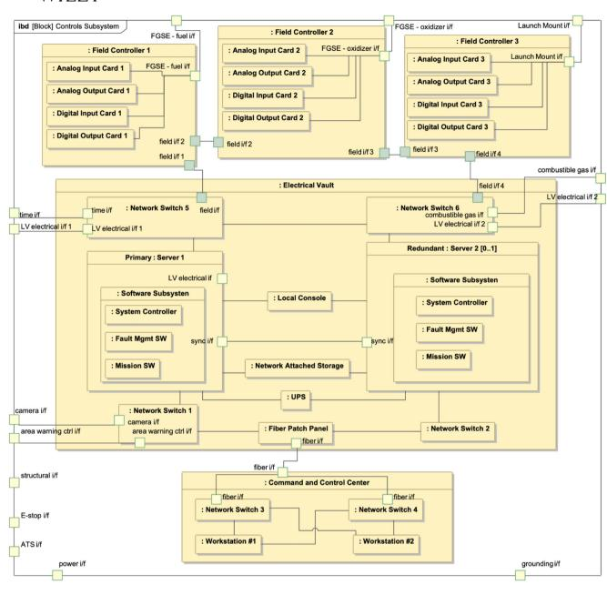
FIGURE 4 Control subsystems IBD (Level 3)
