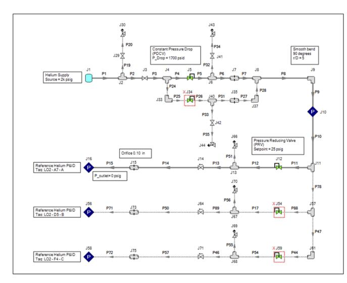
FIGURE 6 AFT arrow FGSE helium fluid dynamic model configuration
