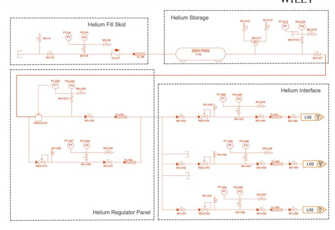
FIGURE 5 P&ID for FGSE helium subsystem
