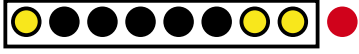
Fig. 1: The nearest neighbors to a test instance (with k = 3 ). The red point represents the unlabeled instance and the yellow ones are the nearest neighbors in the window according to a distance metric.
