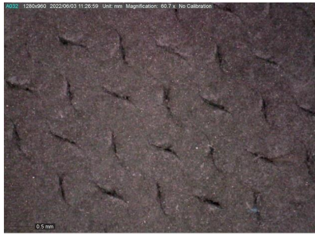
Figure 81 - Gyroid microstructure non-sintered cube
