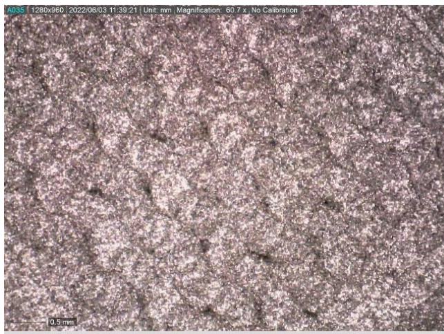
Figure 82 - Gyroid microstructure sintered cube
