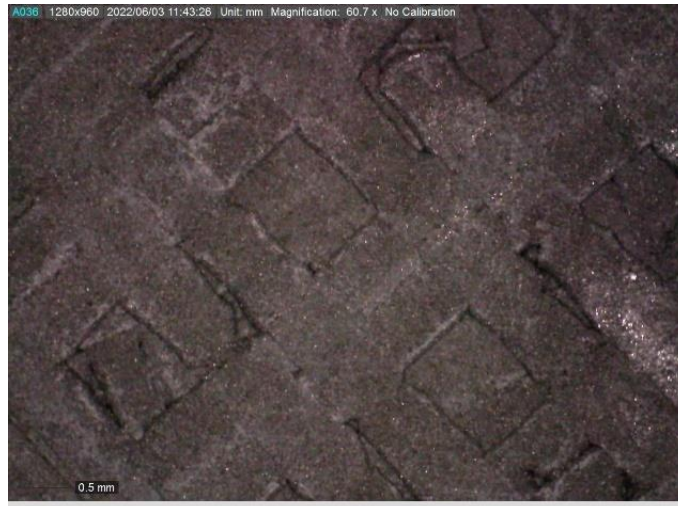
Figure 85 - Quarter cubic microstructure non-sintered cube
