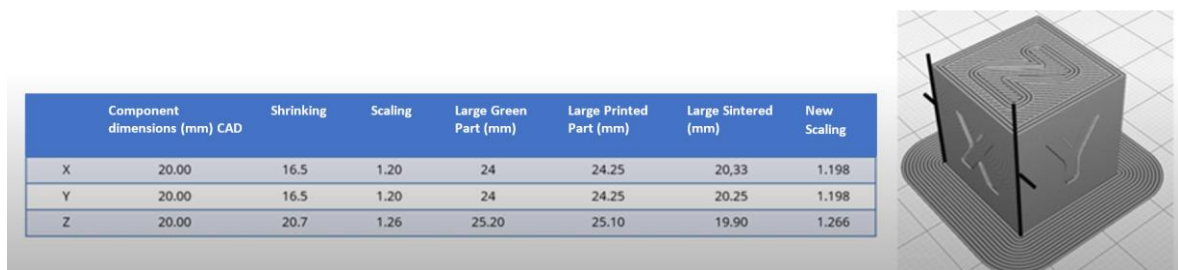
Figure 50 - Percentage recommended for the BASF because of shrinkage (IGO3D, 2020)
