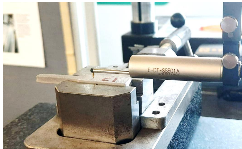
Figure 73 - Surface roughness test
