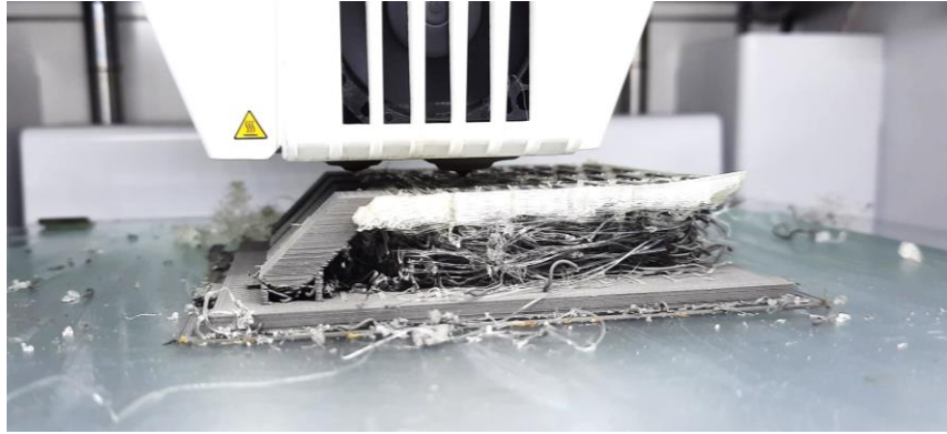
Figure 64 - Printing of the 45° specimens failed
