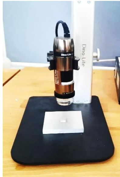
Figure 71 - Dino-Lite microscope for microscopic analysis
