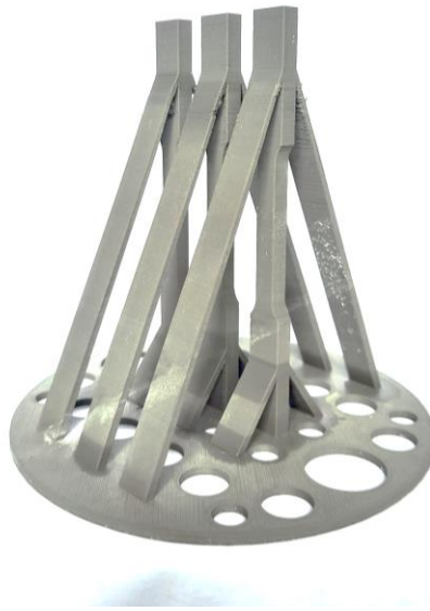
Figure 67 - 90° specimens with two supports
