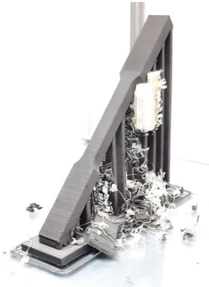
Figure 65 - 45° specimen printed with PVA structures
