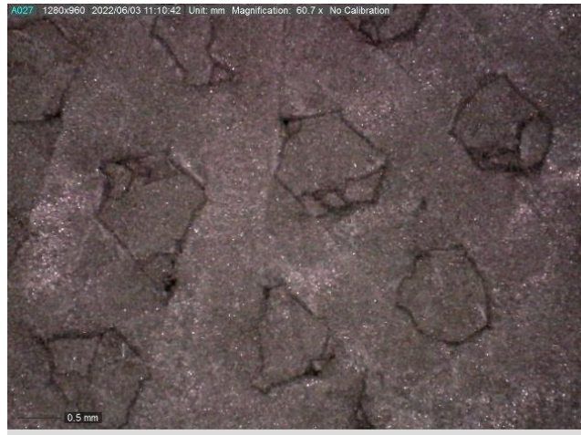
Figure 83 - Tri-hexagon microstructure non-sintered cube
