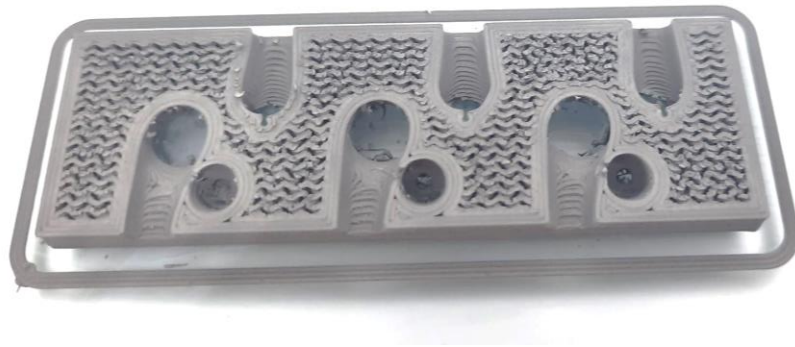
Figure 99 - Car cylinder head being printed
