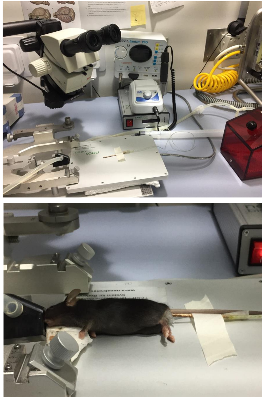
Figure 2.7: Electrocautery surgical setup: Top image shows the surgical microscope, electrocautery machine, dental drill, heated surgical pad and stereotaxic instrument. The bottom picture shows an anaesthetised mouse with the head in the nose cone at a 30° angle; the mouse also has the rectal temperature probe in place for the feedback control of the heated surgical pad.
