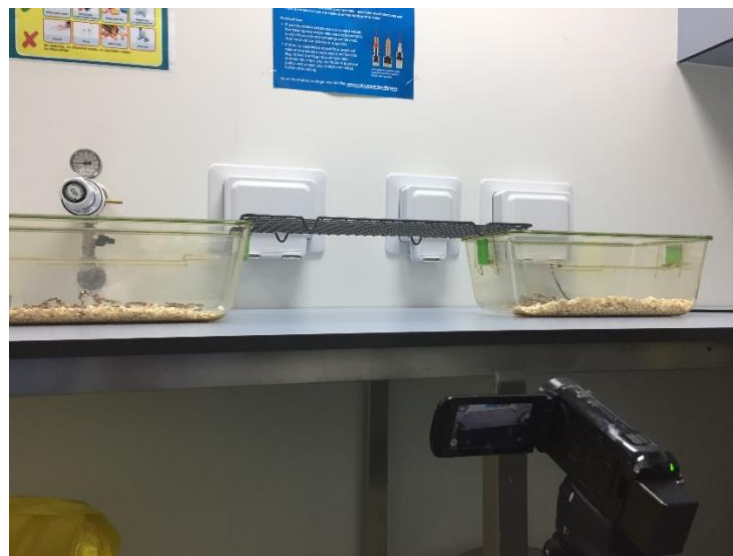
Figure 2.14: Recording setup for the grid walking test: The grid is set on top of two cages, and the video is shot from below.
