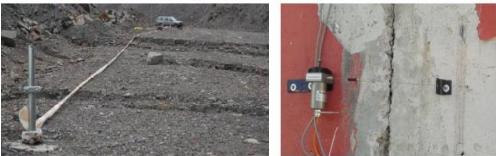
Figure 3. 8 Extensometer in action (10)
