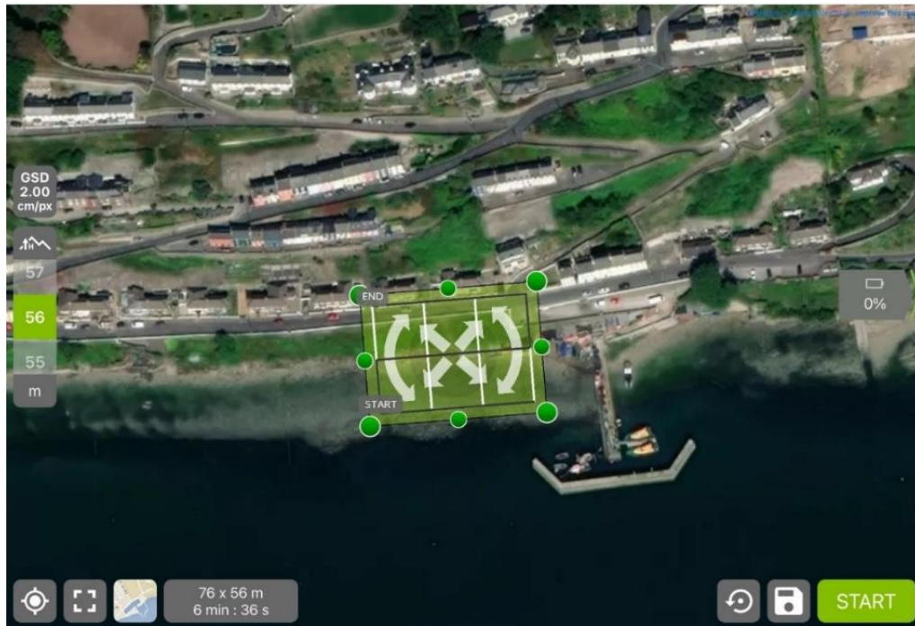
Figure 4. 20 Selection of the area to be flown by the drone over the Connolly Street slope, Cobh
