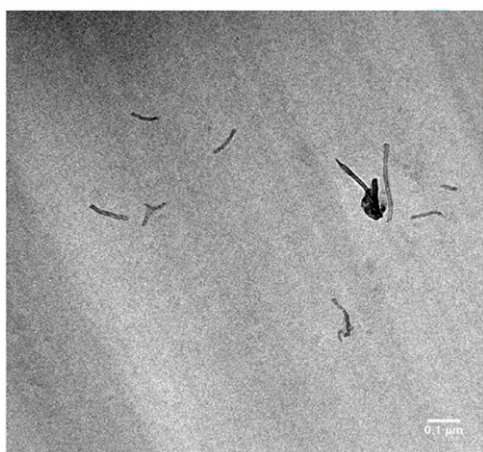
Figure 5. Transmission electron microscopy image of CNTs within PPSU tufting yarn at an accelerating voltage of 200 kV.
