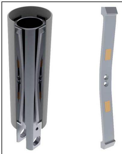
Figure 6. Low-cost force sensor based on a flexural system formed by four lever opposed couples distributed at 90^\circ (left). Detail of strain gauges placement on one lever (right).
