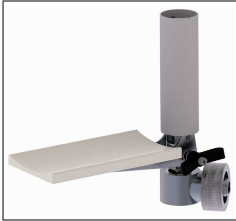
Figure 5. Detachable end-effector with two passive DOF.
