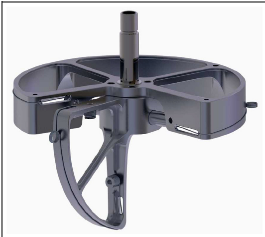
Figure 4. HomeRehab pulleys and cable transmission system.
