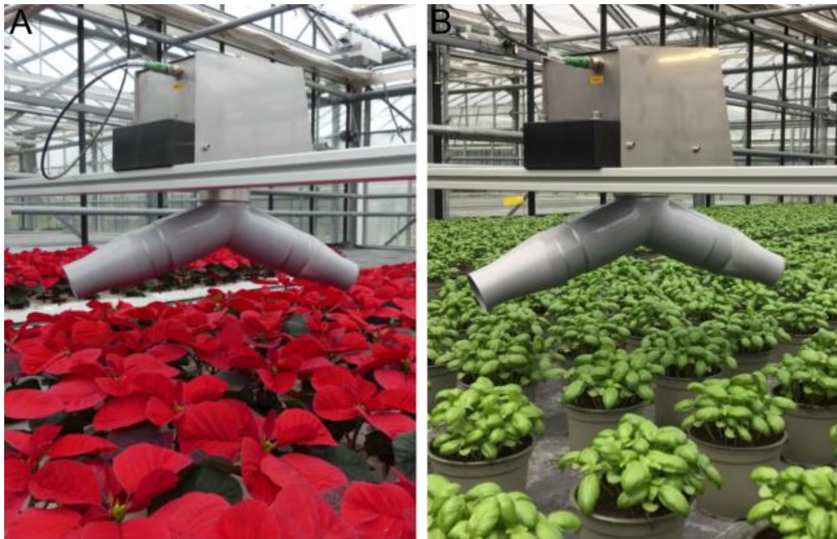
Fig. 7.3. The new prototype (Raith Tec, Ditzingen, Germany) was installed at the State Horticulture College and Research Institute, Heidelberg, Germany for growth control by air stream-based mechanical stimulation of poinsettia (A) and basil (B).
