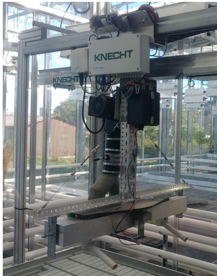
Fig. 5.1. The air stream applicator installed at the University of Hohenheim, Stuttgart, Germany.
