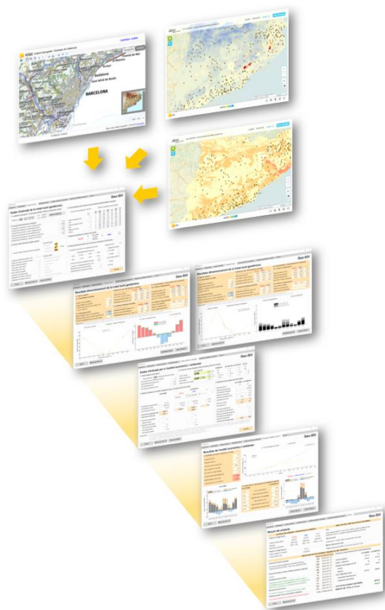
Figure 2: Geo-SIV loads geological data according to the location specified by the user automatically, prior to the size, simulation and economical and environmental analysis of the SGE installation.
