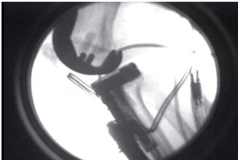
Figure 2. 1. Prosthesis relevant to the analysis, incorporating sensors for the measurement of contact forces [6].
