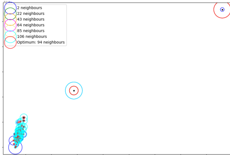
Figure 17: Representation of the LOF system. The circumferences surrounding each data point (black) represent the LOF score, so higher radiuses mean higher scores. Each circumference color represents scores from different k-neighbors, ranging from 2 (minimum for this system to work) to 106 (total number of points). The optimum value for k-neighbors (red) gives the higher scores to the 2 furthest points, assigning the higher score to the most extreme one.
