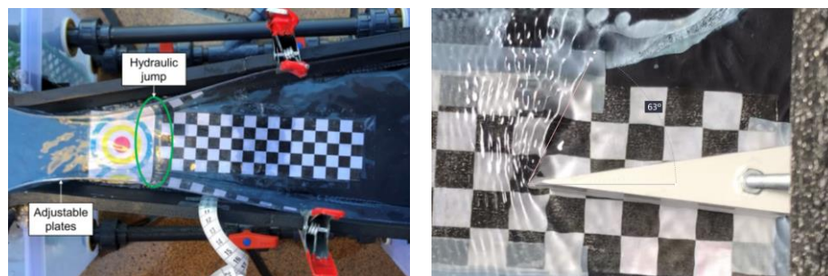
Figure 2. Left) Photographic capture of a hydraulic jump; Right) Photographic capture of obliquity
