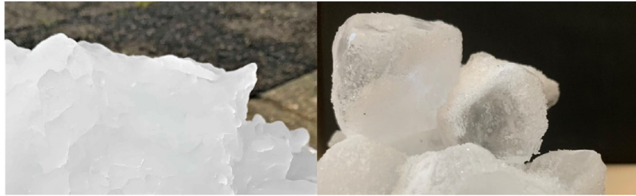
Fig. 1. Liquid ice can be seen on the left side and block ice on the right.
