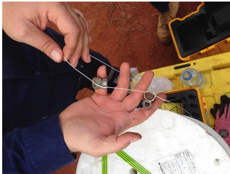
Figure 3-13. Details from the field experiment – tight buffer FO cable deployment.
