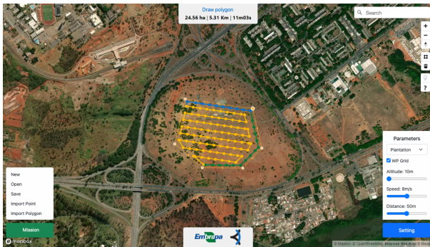
Fig. 2: Application Interface for CPP with UAV
