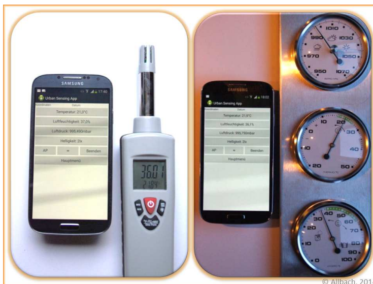
Fig. 4: Samsung Galaxy S4 vs. common measurement devices.
