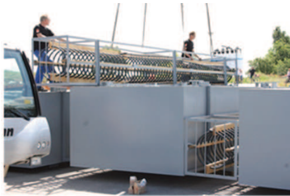
Fig. 14: Process of constructing of two spirals- heat exchanger between of three parts of pontoons, Fig. 15: Simulation of heat- mass transfer processes in spiral underwater heat exchangers in software ANSYS FLUENT 13.0
