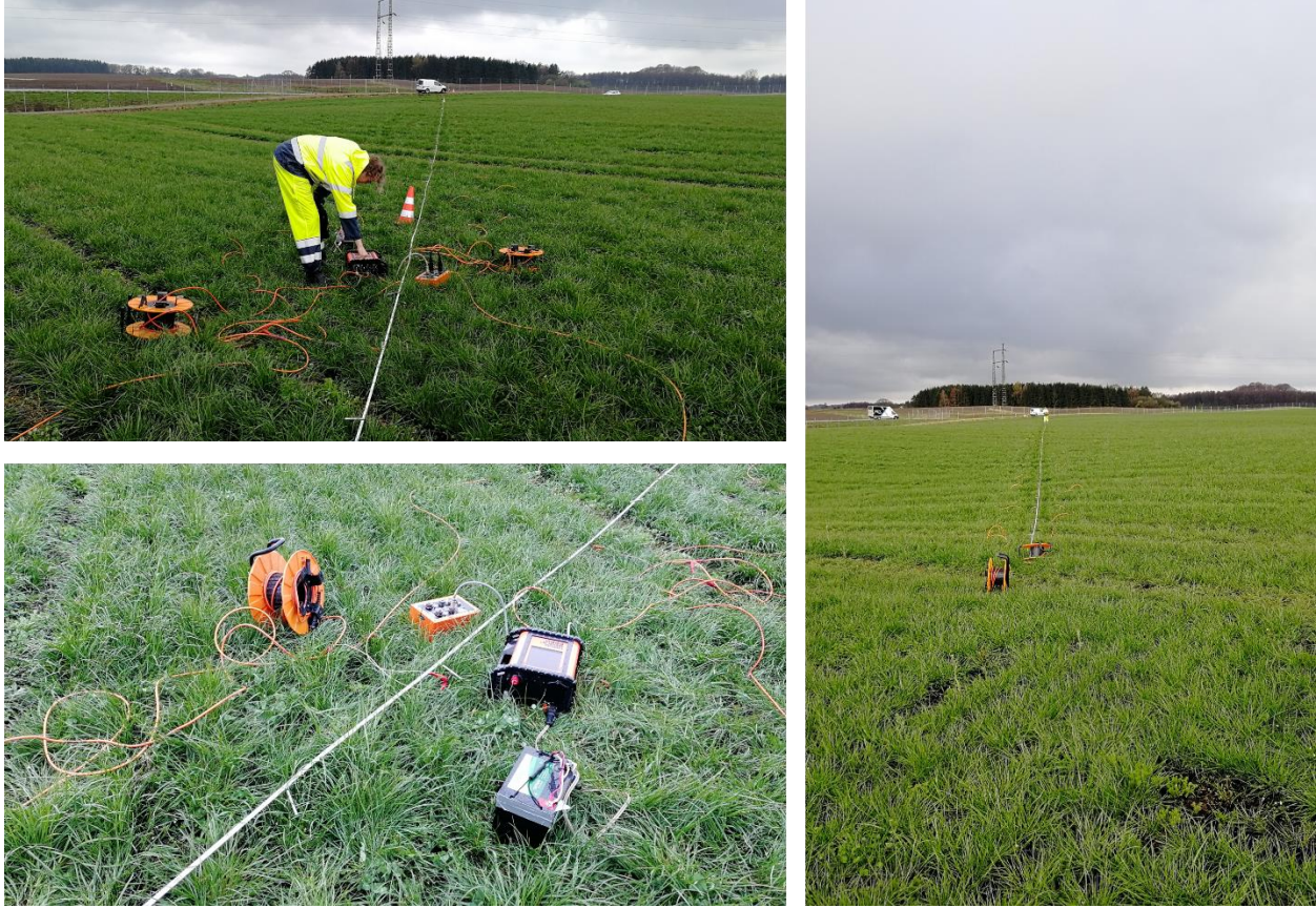
Figure 1: DCIP field setup with the different multi electrode cables and the ABEM Terrameter LS2 instrument.
