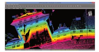
Fig.17: LIDAR from terrestrial scanning are excellend data source for buildings elevation details
