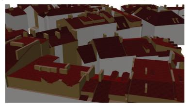
Fig.13: sample model 3D, CityGML LoD 2, with roof details from stereodigitizing
