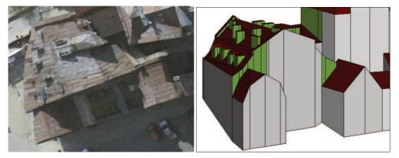
Fig.15: source data(aerial), Fig.16: Model 3D derived from stereodigitizing
