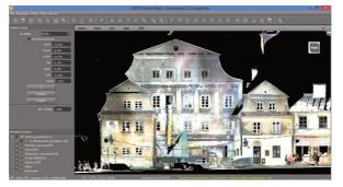
Fig. 18. Result of terrestrial laser scanning, PTS format (z,y,z + color data), scan by LEICA P20
