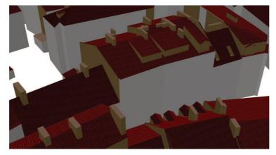
Fig.14: sample model 3D, CityGML LoD 2, with roof details from stereodigitizing
