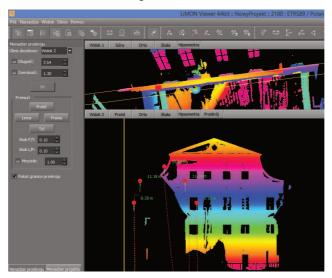
Fig.20: 3D data of terrestrial laser scans are ideal complementary data source for aerial scannning or data derived from stereodigitizing of aerial photos.
