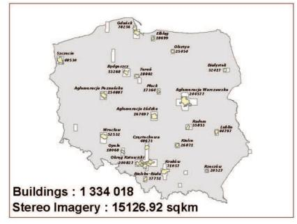
Fig. 2 : Collection of IKONOS satellite srereopairs for 42 cities of Poland by SCOR SA, resulted in acquisition of 15 126,92 km², what allowed for construction of simplified 3D models of 1 334 018 buildings in 2005
