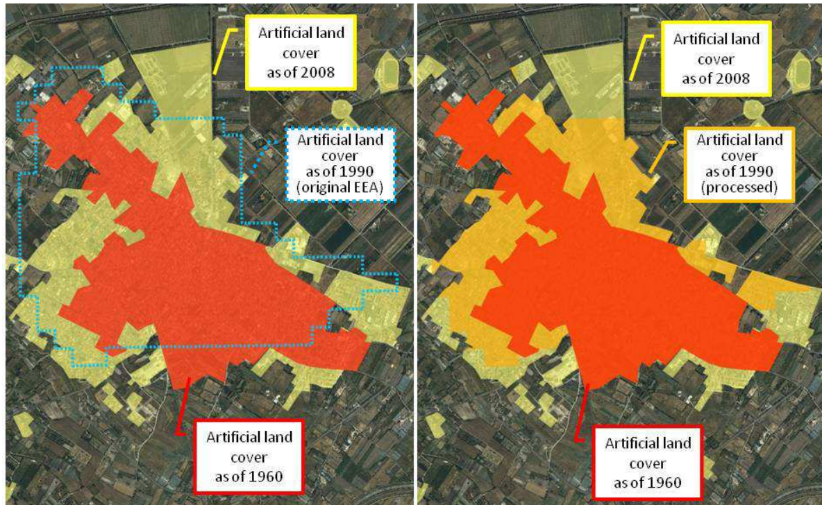
Figure 1: Analysis of changes in artificial land cover between 1960 and 2008: an example showing correction of inconsistencies due to differences in map resolutions.
