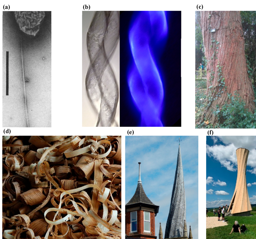
Figure 6. Chirality of cellulose and cellulosic materials. (a) Chiral twisting of a single fibril of bacterial cellulose (image has been rotated for clarity, and scale bar = 1 \mu\text{m} ). 84 (b) Twisting of cotton fibers (image courtesy of R. M. Brown). (c) Image of a twist in the trunk of Eucalyptus gigantea (photograph taken in the grounds of Exeter University (S. J. Eichhorn)), (d) Twisted wood shavings (CC-BY image). (e) The twisted spire of Chesterfield church, UK (CC-BY image), and (f) the Urbach tower in Baden-Württemberg, Germany (CC-BY image).
