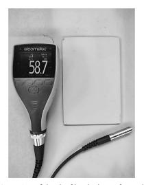
Figure 2 Measuring of the dry film thickness formed by the primer with the dry film thickness of 60 μm
