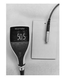
Figure 3 Measuring of the dry film thickness formed by the primer with the dry film thickness of 45 μm
