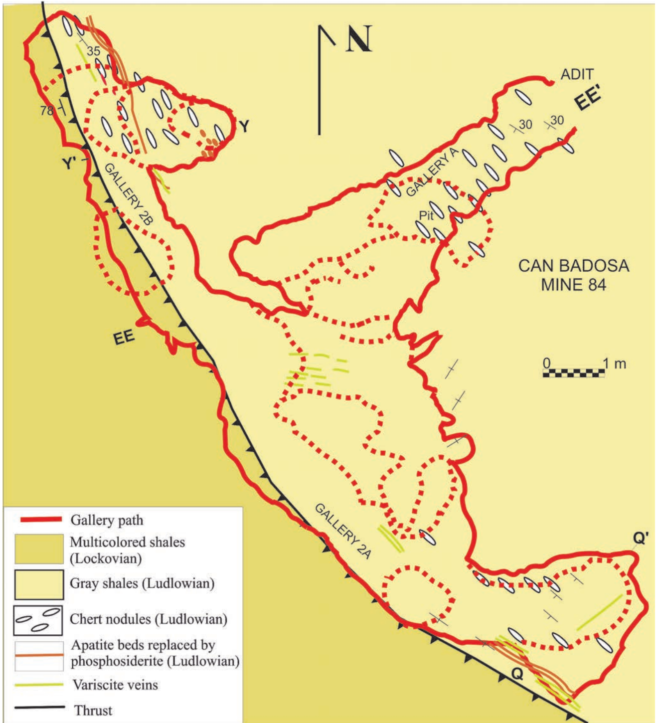
Figure 11 Topography and geological map of mine 84 at Can Badosa, showing the distribution of the mineralized units and the location of sections shown in Figure 12. Modified after Melgarejo et al. (2009).
