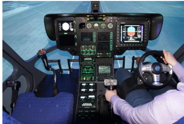
**Figure 9.** Steering wheel control for a personal aerial vehicle [44].
