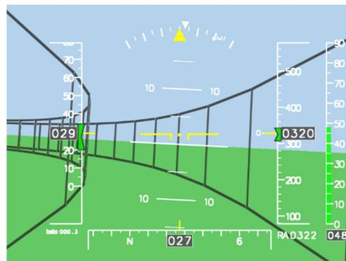
**Figure 10.** Highway-in-the-sky concept as navigation assistance for minimally trained pilots [46].
