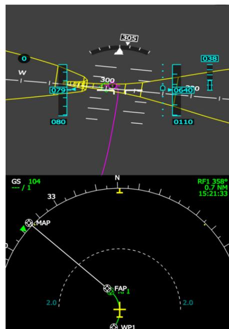
Figure 4. Synthetic vision system with tunnel-in-the-sky display.
