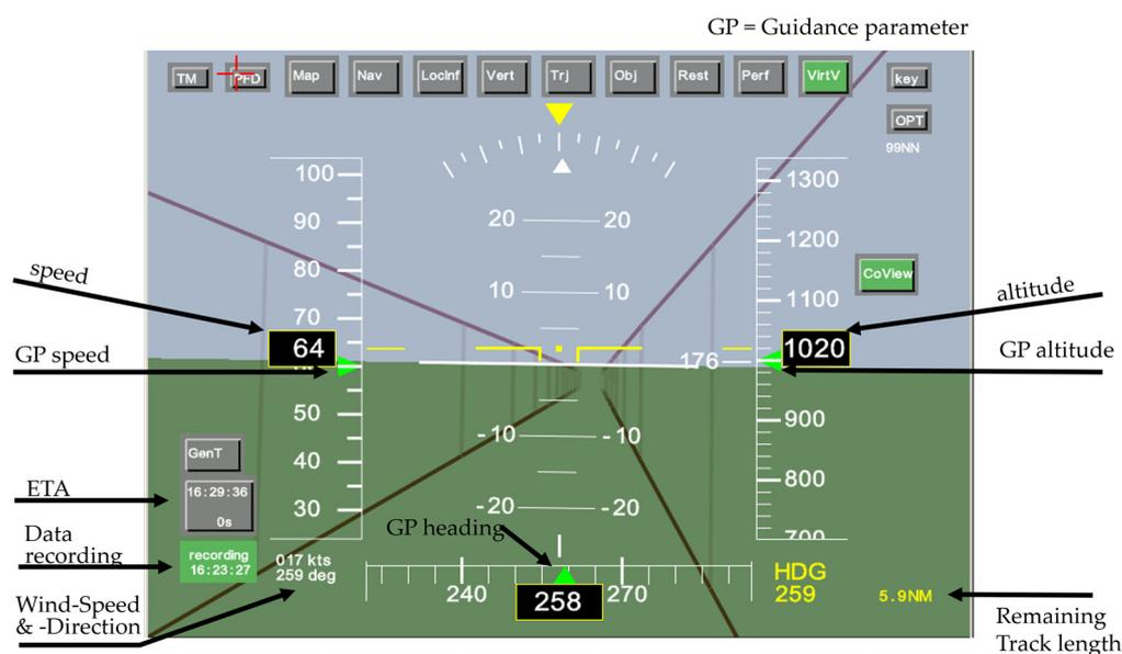
**Figure 2.** Tunnel-in-the-sky display (dark purple lines) and overlaid Bug-PFD-guidance display.
