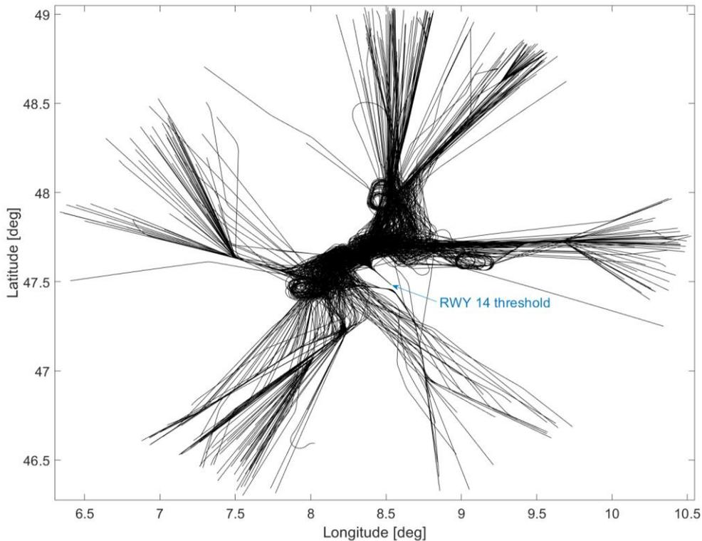
Figure 1 – Lateral flight paths (top view of ground tracks) of all 667 Airbus A320 flights into Zurich airport investigated for the analysis. The depicted tracks begin at Flight Level (FL) 100 and end at the threshold of the target runway 14, which can be seen in the centre of the figure.
