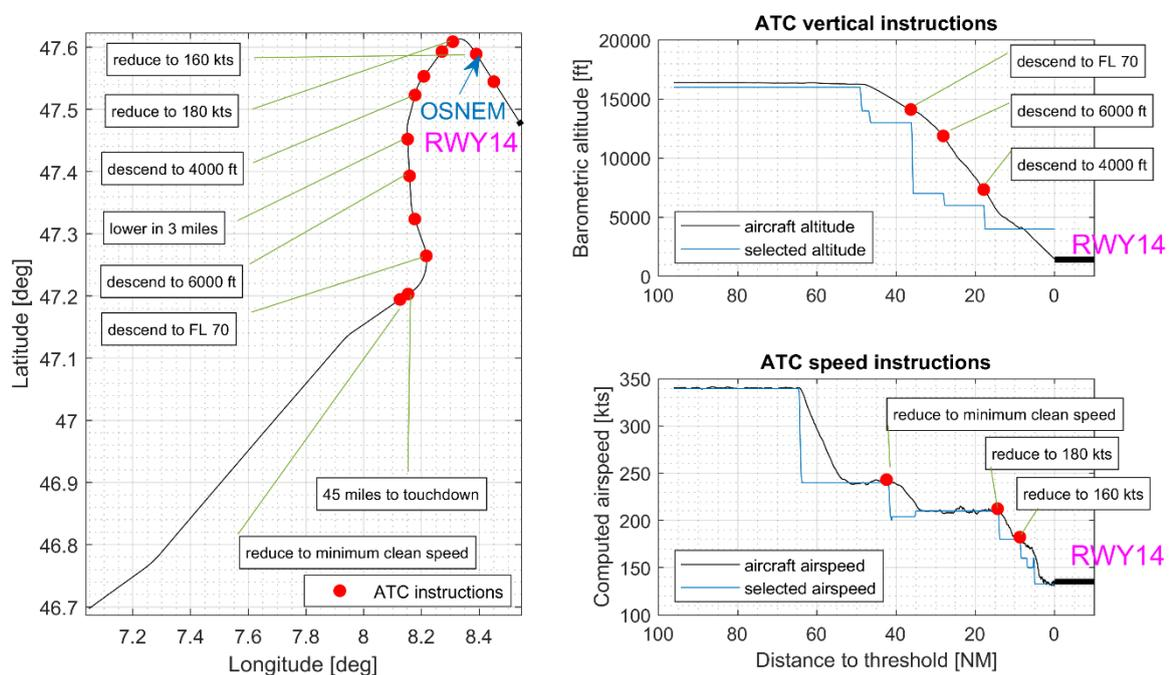
Figure 3 – Sample evaluation for flight #41 of 667, illustrating ATC instructions to the aircraft over lateral profile (left); vertical (upper right) and speed (lower right) instructions and the respective resulting profiles flown. OSNEM is the Final Approach Point (FAP) for runway 14.
