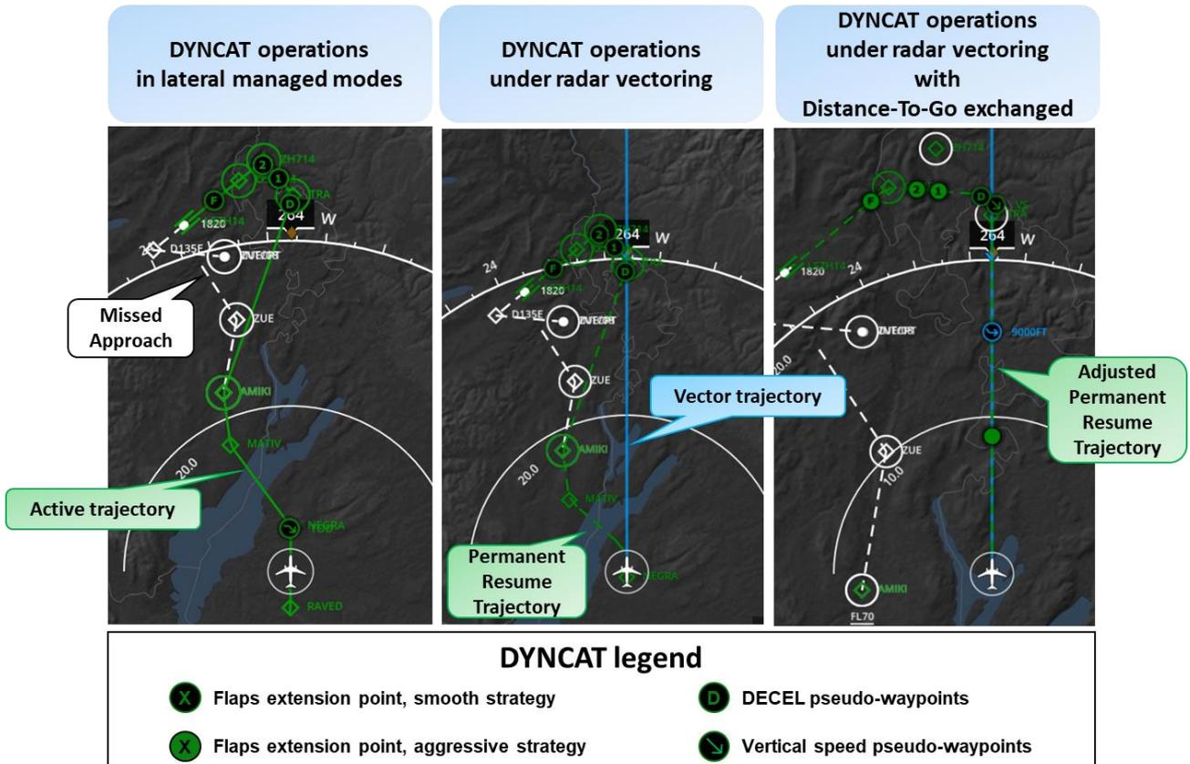
Figure 4 – DYNCAT flight plan depiction on Navigation Display in typical chronological order: initially managed mode displaying published transition (left); then selected mode employed under radar vectoring, before (middle) and after (right) reception of DTG information. The active trajectory or PRT, resp., are the reference for calculation of the pseudo waypoints for configuration and airspeed / vertical speed changes.
