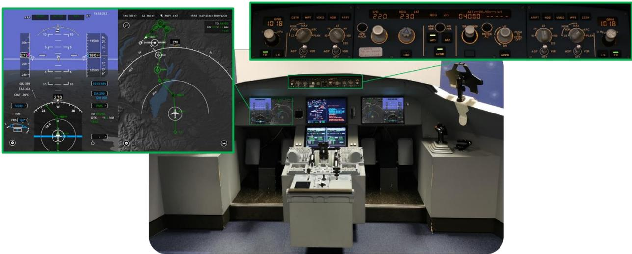
Figure 5 – Flight test simulation bench (Thales, Toulouse) with new generation Cockpit Display System (upper left, comprising ND and PFD) and A320 family Flight Control Unit (upper right)
