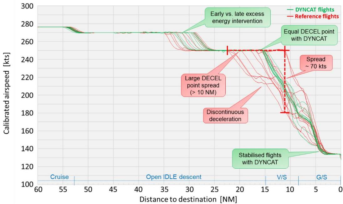
Figure 8 – Speed profiles from piloted simulations, 12 without (reference, red) and 12 with the DYNCAT functionality (green). (V/S: vertical speed segment; GS: glideslope segment)
