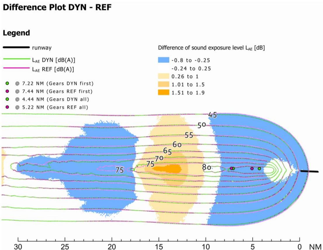
Figure 11 – Differential plots (DYNCAT and reference; colour coded blue and orange) and noise contours (green and purple, resp.) of calculated sound exposure level  $L_{AE}$  at the ground for straightened trajectories. The ground is assumed flat and acoustically soft (grassland). The filled circles denote the respective earliest and latest landing gear extension points.
