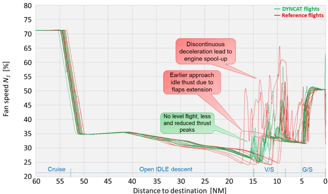
Figure 9 – Engine fan speed  $N_1$  (expressed as percentage of maximum normal rotational speed, indicating thrust level) from piloted simulations, 12 without (reference, red) and 12 with the DYNCAT functionality (green). (V/S: vertical speed segment; GS: glideslope segment)
