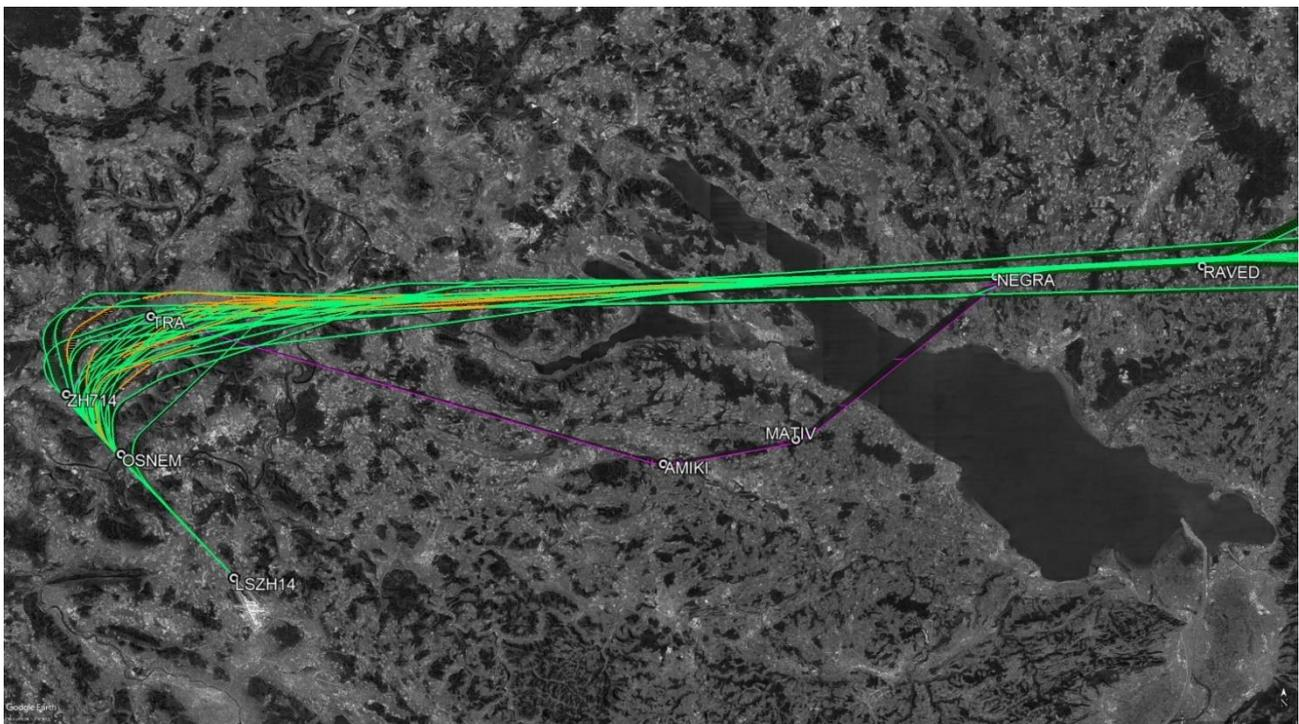
Figure 6 – Real flight trajectories selected as reference for piloted simulation scenarios. Those trajectories represent over-energy situations caused by a shortcut against the published transition (reference flight plan, depicted in purple) starting from NEGRA waypoint. OSNEM is the FAP, LZSH14 the runway threshold. (credit: Google Earth)
