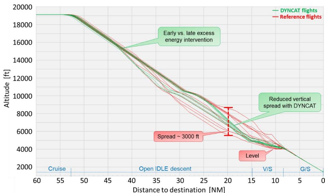
Figure 7 – Altitude profiles from piloted simulations, 12 without (reference, red) and 12 with the DYNCAT functionality (green). (V/S: vertical speed segment; GS: glideslope segment)
