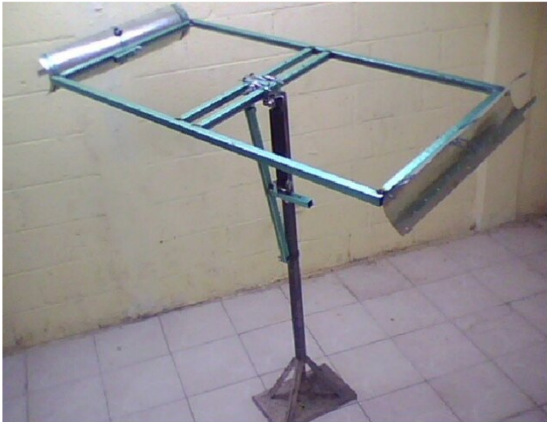
Photo 7.2.2 A bi-metallic actuated single axis platform
