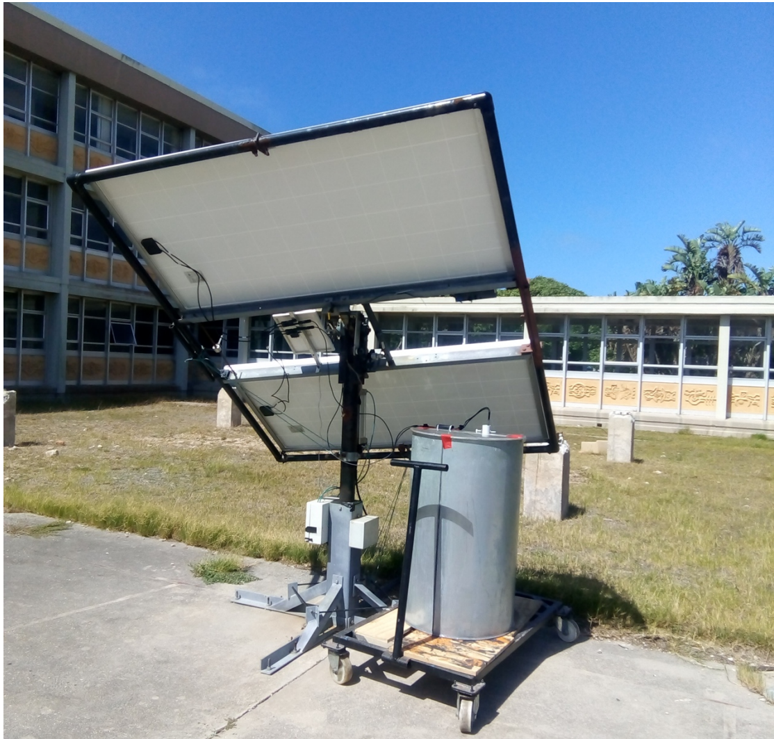
Photo 12.6 Prototype test rig with water tank heat sink
