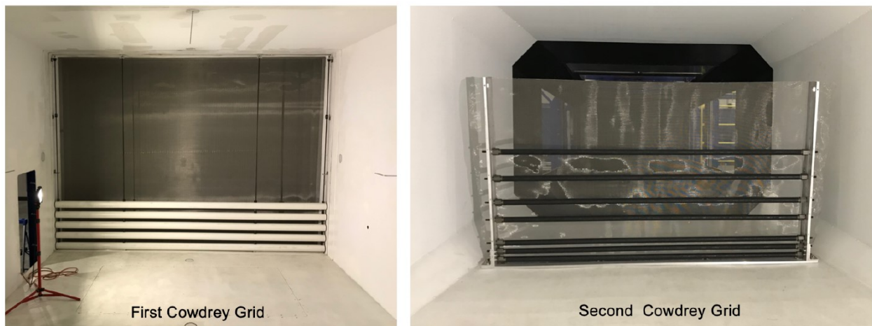
Figure 2.3 Two sets of Cowdrey grids in the LSWT facility used in the present study [14].
