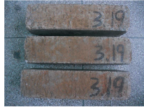
FIGURE 3: Appearance damage of specimens N10G1R45 after 90 cycles of drying-wetting.
