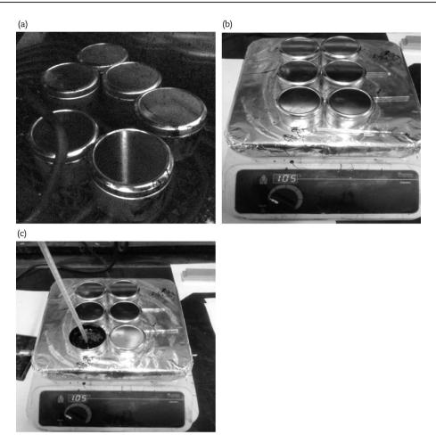
Fig. 2 — Test procedure. (a) Asphalt binder preheated in an oven for at least 90 min at foaming temperature. (b) The container placed on a hot plate to avoid temperature reduction due to room temperature. (c) Measurement of temperature after binder foaming process.
