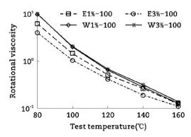
Fig. 10 - Comparison of foamed binders prepared with ethanol and water as foaming agent at 100  $^{\circ}$ C.
