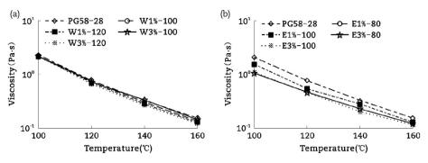
Fig. 6 - Comparison of rotational viscosity of un-aged foamed asphalt binders. (a) Water. (b) Ethanol.
