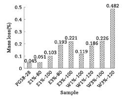
Fig. 7 - Volatile loss of foamed binder using the rolling thin film oven test.
