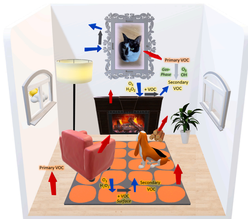
Fig. 1. The chemical processes and transformations following deposition of oxidants on internal surfaces in the indoor environment.
