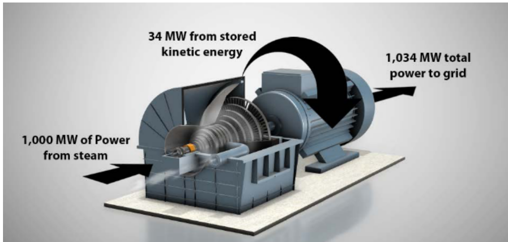
Figure 1.3: When the electrical demand of this synchronous generator suddenly increases, the inertia of the steam turbine and electric generator makes up the shortfall. Reproduced from Ref. [8].
