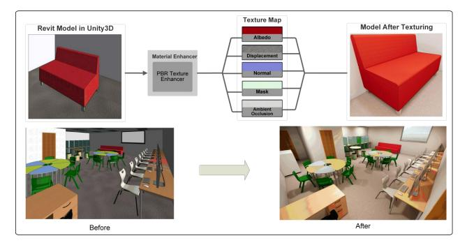
Figure 5.5: Re-Texturing Revit Model in unity using PBR materials (Classroom Model)
