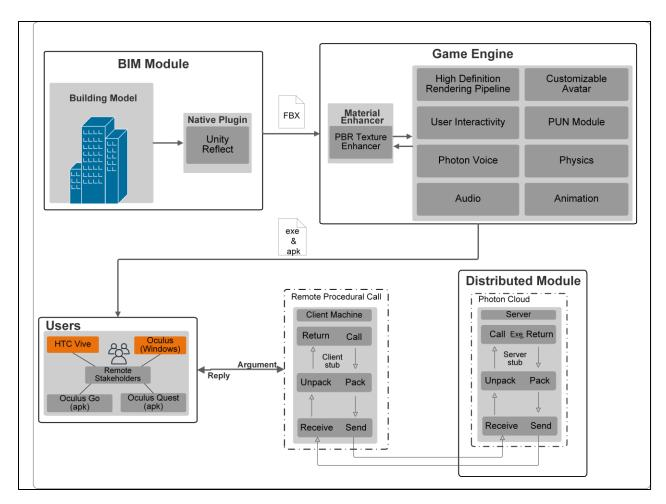
Figure 5.2: System architecture
