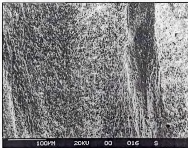
Figure 7.17 Fractograph of R=0.7 CAL at \Delta K = 2.4 \text{ MPa.m}^{1/2} on Ti1023
