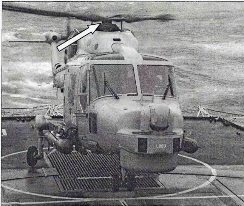
Figure 1.1 Lynx helicopter showing location of the rotorhead used in this investigation. (Courtesy of GKN Westland Helicopters Ltd.)
