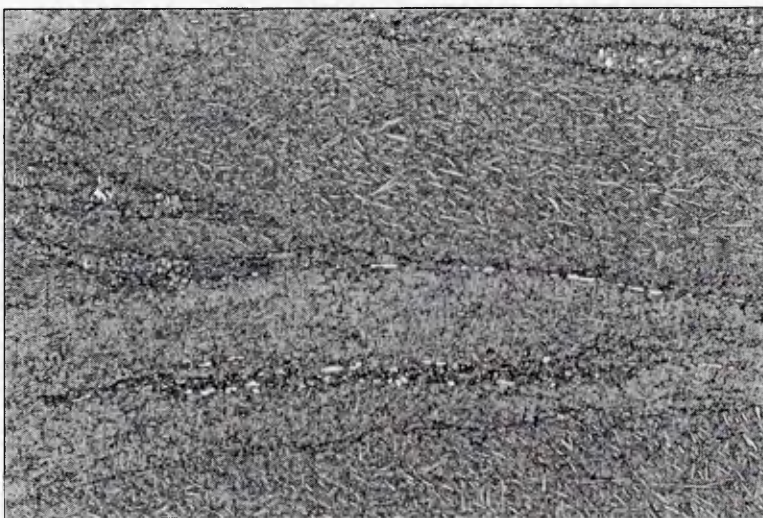
Figure 6.8 Microstructure of Ti-1023 in T-S plane (Mag. x30)
