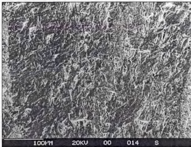
Figure 7.16 Fractograph of R=0.4 CAL at \Delta K = 4.8 \text{ MPa.m}^{1/2} on Ti1023
