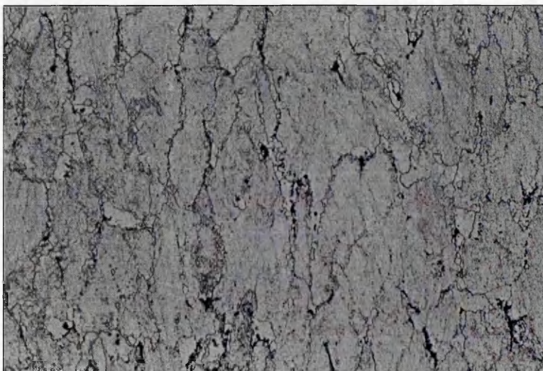
Figure 6.12 Microstructure of 7010 in L-S plane (Mag. \times 30 )
