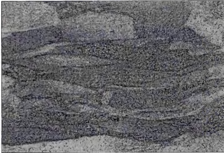
Figure 6.6 Microstructure of Ti-1023 in L-T plane (Mag. x30)
