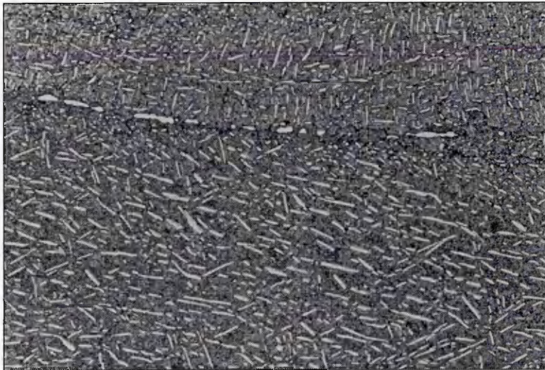
Figure 6.7 Microstructure of Ti-1023 in L-S plane (Mag. x60)
