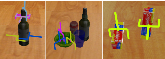
Fig. 6. Examples of grasping objects in different situations: (left) predicted grasp configurations for orthographic views of the object; (center) grasp prediction for a clutter scene that are both kinematically feasible and collision free; (right) the best grasp configuration for grasping a Colgate object in two different situations.
