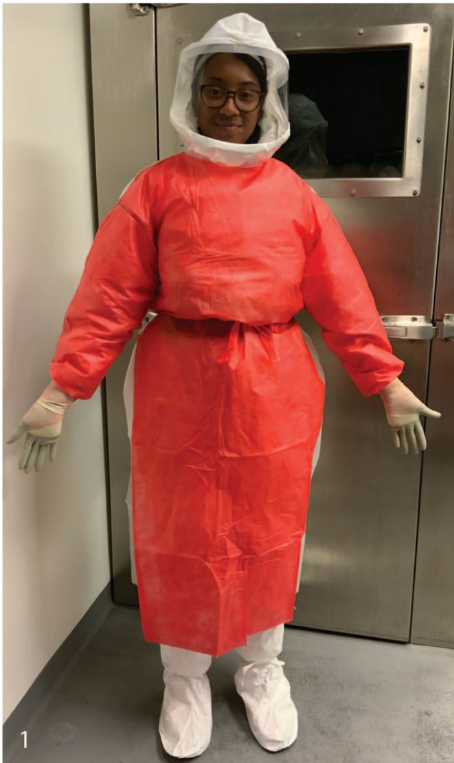
Figure 1. Typical personal protective equipment worn in a BSL3 facility, including powered air-purifying respirator, Tyvek suit, solid-front gown, double gloves, and shoe covers.
