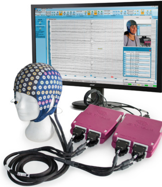
Figure 2.4: Basic EEG setup: EEG cap, amplifier, software and computer. From ANT-neuro, eego TM mylab
