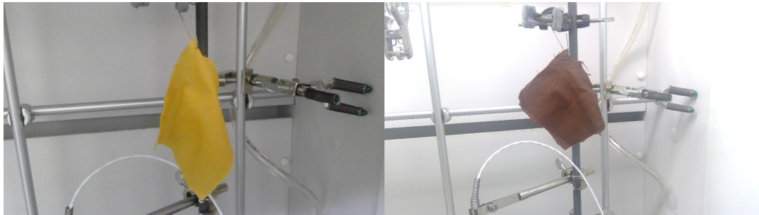
Figure A8. Low load (left) and high load (right) cotton fabrics synthesized by Justin Gorham (NIST). XPS analysis was used to determine the Ag loading: 0.16% for the low load fabric and 0.31% for the high load fabric.
