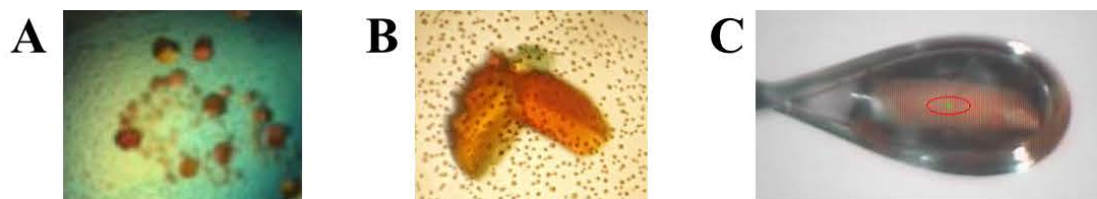
Figure 16. T1-RHPS4 crystals. (A) Initial crystallization hit by Irene Xiang '18 in HELIX condition 1-31. (B) Optimized crystals that yielded one of the best datasets. (C) Looped crystal being shot with an X-ray beam at the synchrotron. Crystals are shown at approximate relative sizes.
