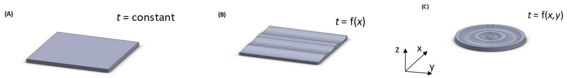
Figure 1- Types of sheets that can be used: (A) constant thickness; (B) spline thickness variation on x-direction and (C) concentric thickness variation (adapted from [2] under an open access Creative Common CC BY license).
