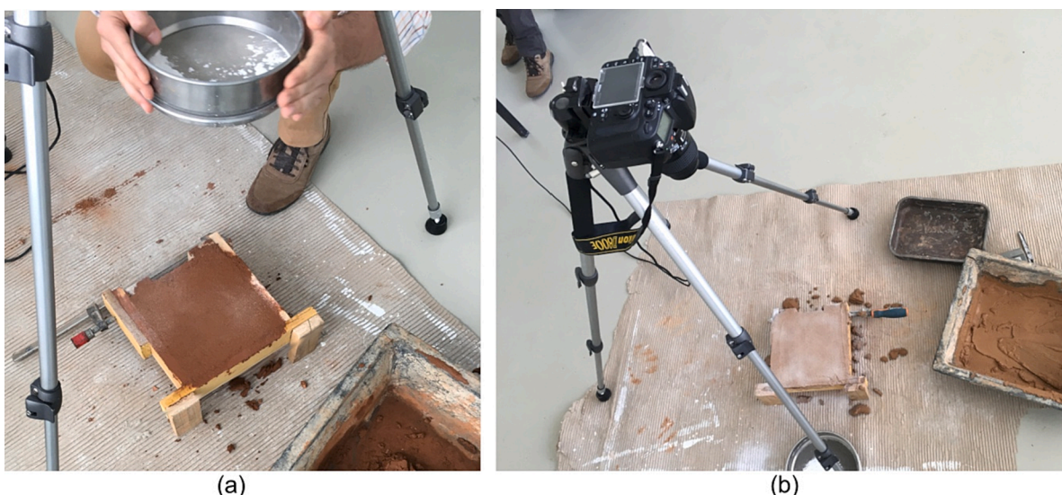
Fig. 3. Third preliminary calibration trial: (a) application of the limestone powder (b) testing setup.
