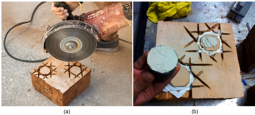
Fig. 6. Preparation of the specimens for the pull-off tests: (a) process used for isolating the cores with octahedral shape.; (b) bonding of the steel plates with epoxy resin.
