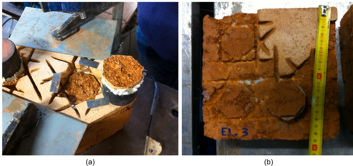
Fig. 14. Failure modes observed in the puff-off tests: (a) example of failure at the interface LC-TRM–substrate, showing a slim superficial layer of the substrate attached to the mortar; (b) large regions of the plaster detached during the experiments.
