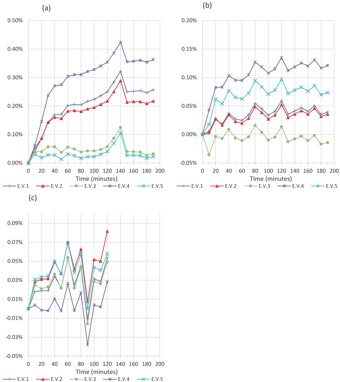
Fig. 9. Strains by Digital Extensometer for all specimens with application of the mortar EM2.0: (a) PE-U; (b) PE-G2; (c) PE-G8.
