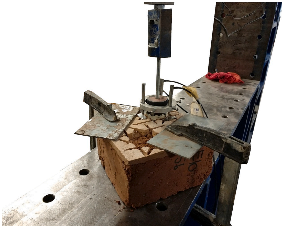
Fig. 7. Testing setup of the pull-off tests.
