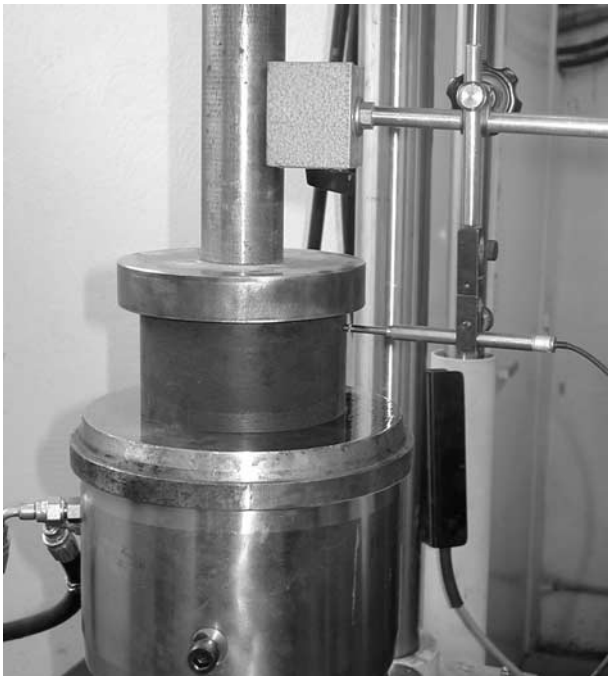
FIG. 5—Photograph of the test device, including the LVDT used to measure transversal displacements during compression.
