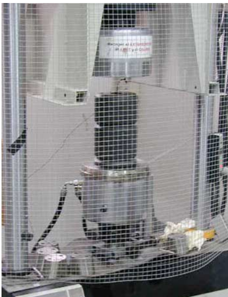
FIG. 2—Photograph of the experimental arrangement to test the buffer under quasi-static uniaxial regime.
