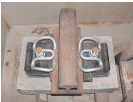
FIG. 14—Fastening system before exposure to salt fog.
