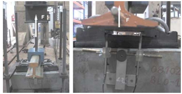
FIG. 8—Clamping force test. Detail of the gap between the foot rail and rail pad during the test.
