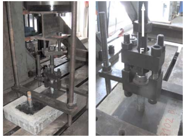
FIG. 11—Testing of embedded components device.
