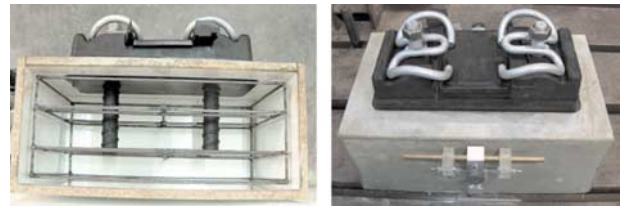
FIG. 4—Manufacture of concrete blocks. Side and top views.
