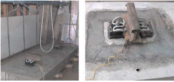
FIG. 13—Electrical resistance test. General appearance and details of electrical connection.
