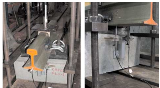
FIG. 5—Dynamic stiffness test at low frequency and detail of the LVDT's location.
